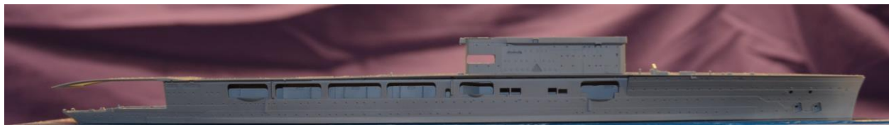
----- Dry-fitting of decks and main island piece -----
